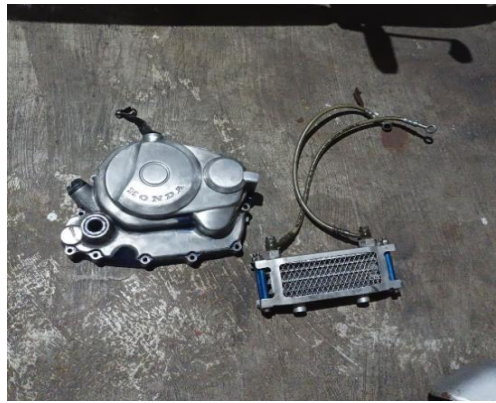
Gambar 2 Jalur oil cooler
